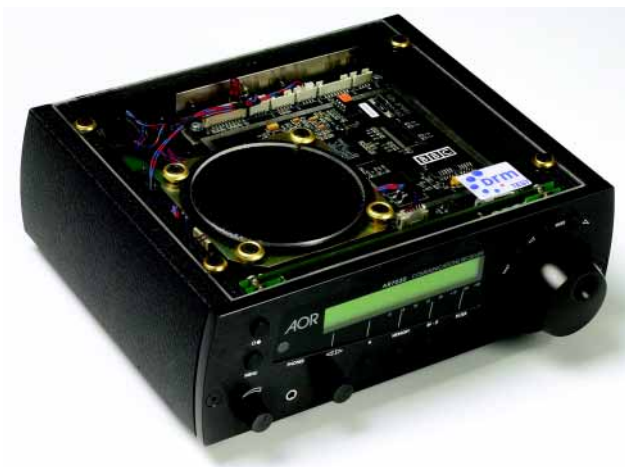
Figure 13 AOR 7030 communications receiver, modified by BBC R&D with the addition of an IF down-converter (see Fig. 5) and the BBC decoder PCB to enable DRM reception.
