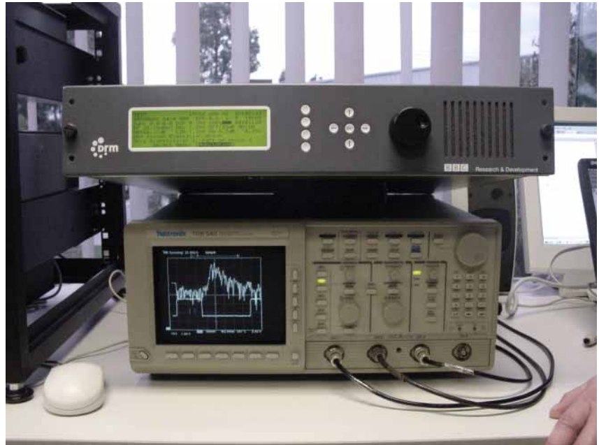
Figure 10 BBC R&D DRM receiver ( top ) with an oscilloscope ( below ), displaying the channel impulse response time, referenced against the symbol period and guard interval
