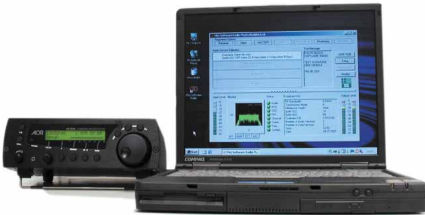
Figure 4 FhG software receiver with modified AOR 7030 receiver (on the left) and a PC running DRM receiver software
