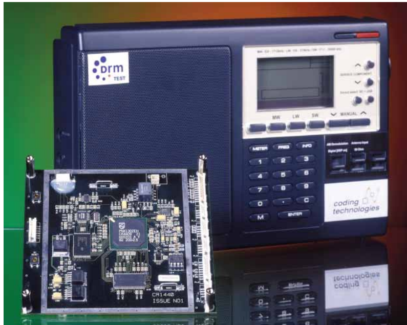
Figure 12 Prototype DRM consumer receiver, manufactured by CTS in association with AFG and BBC R&D. The BBC DRM decoder PCB is shown leaning against the front of the receiver.
