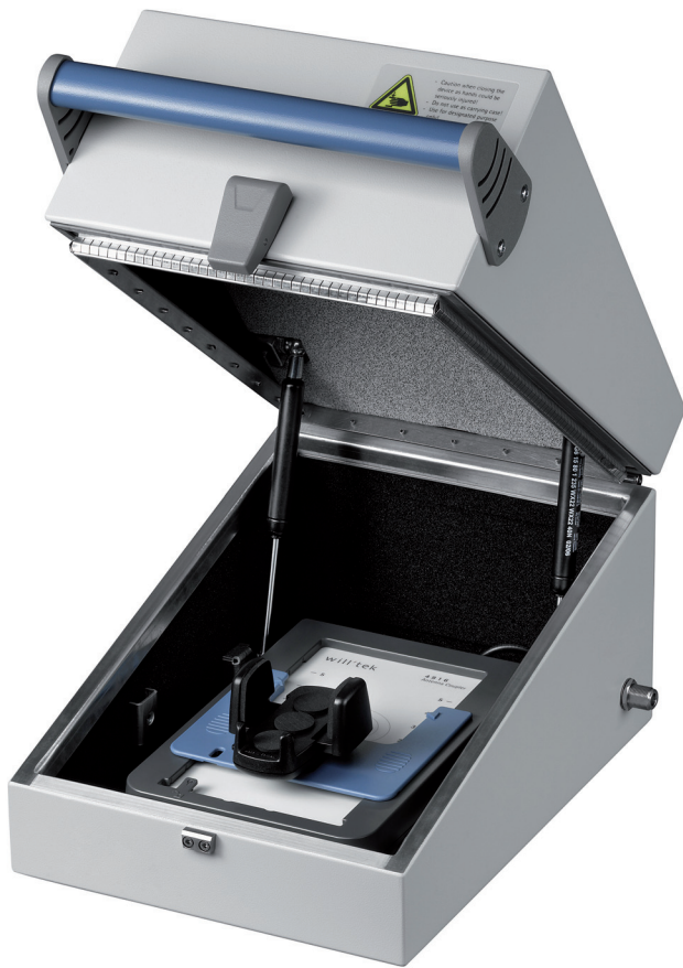
Figure 6: TETRA test chamber with aerial coupler
